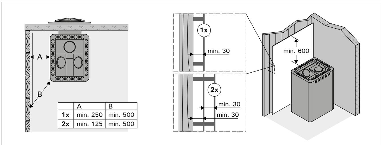
Figure 6. Protective covers (all dimensions in millimeters)
