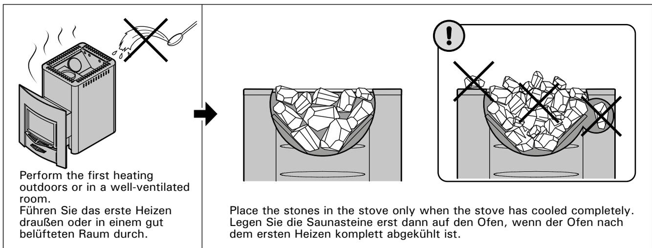
Figure 2. *Preparing the stove and piling the stones*
