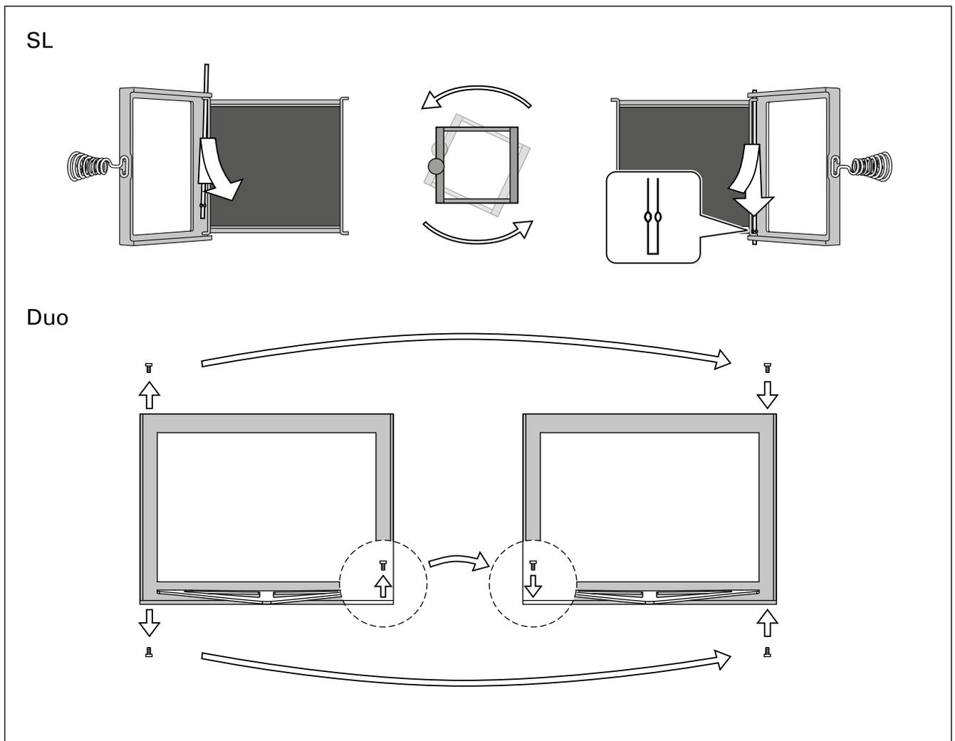
Figure 9. Changing the opening direction of the stove door
