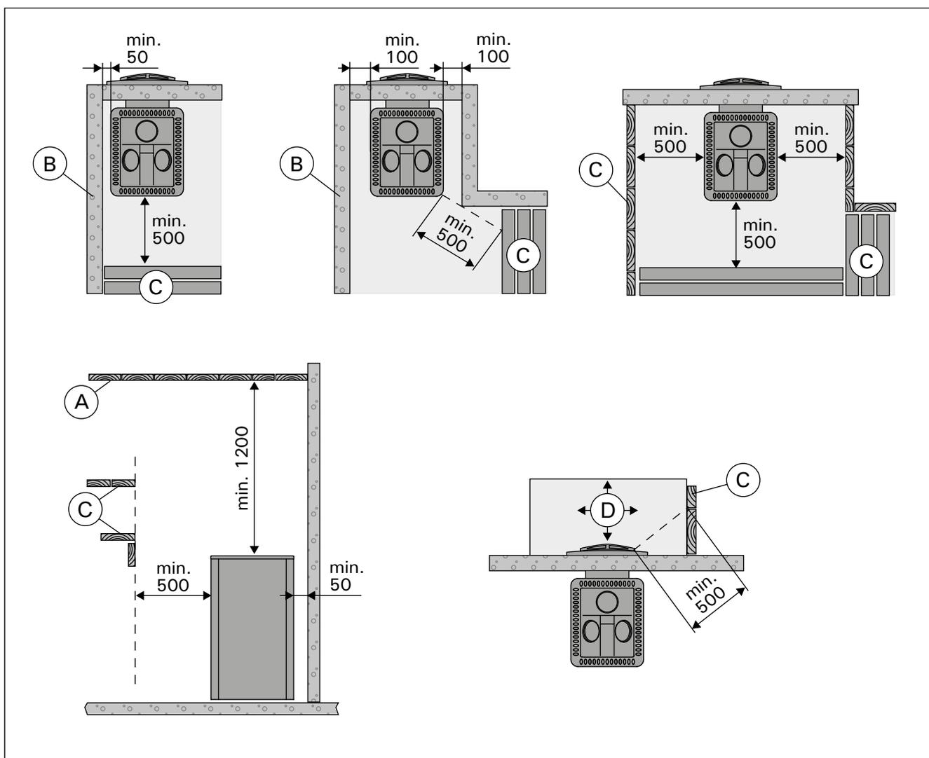
Figure 5. Safety distances (all dimensions in millimeters)
