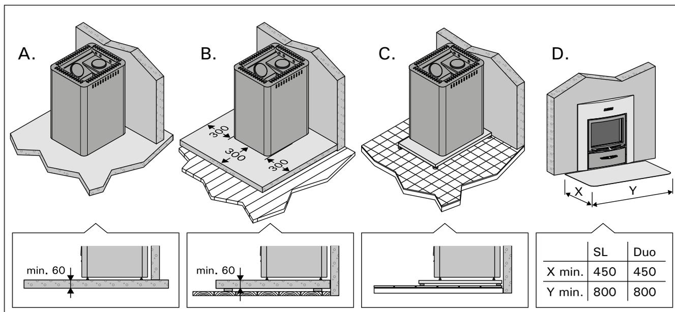
Figure 4. Protecting the floor (all dimensions in millimeters)
