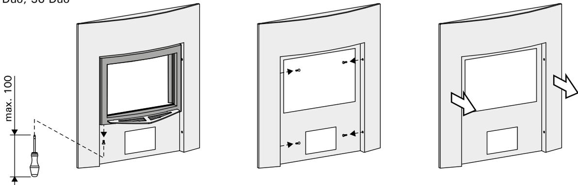
**Figure 7. Installing the stove (all dimensions in millimeters)**
