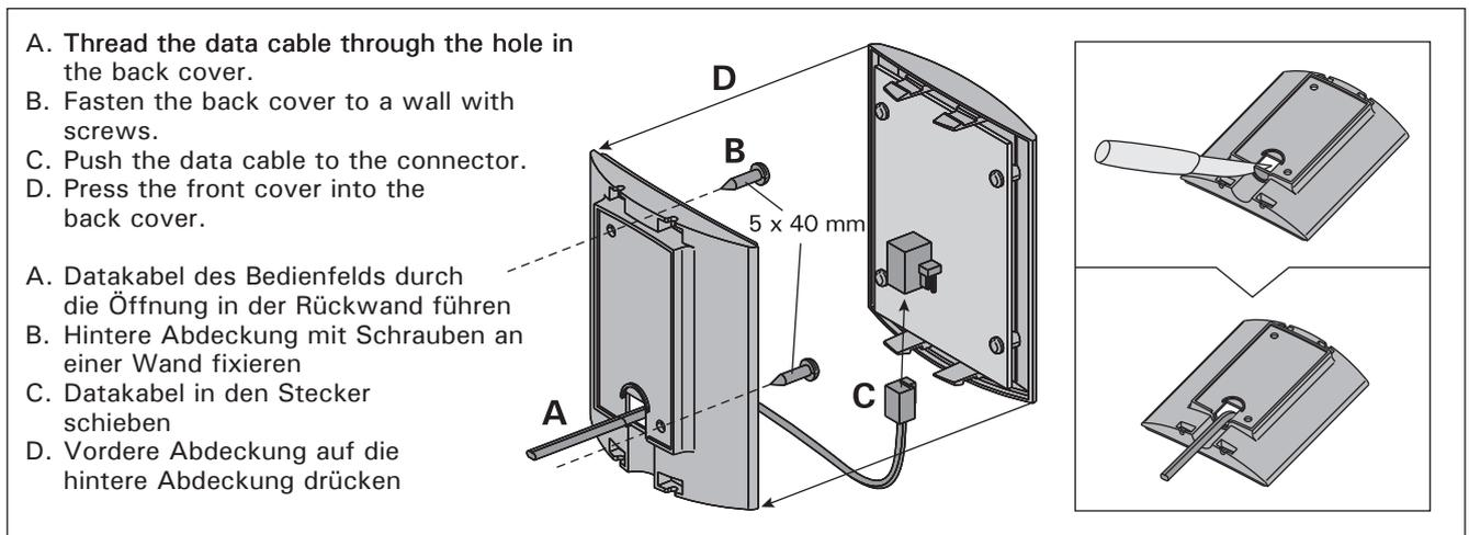
Figure 4. Fastening the control panel
