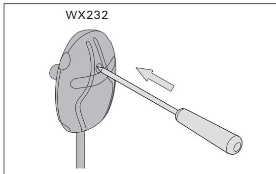
Figure 11. Reset button of the overheat protector
