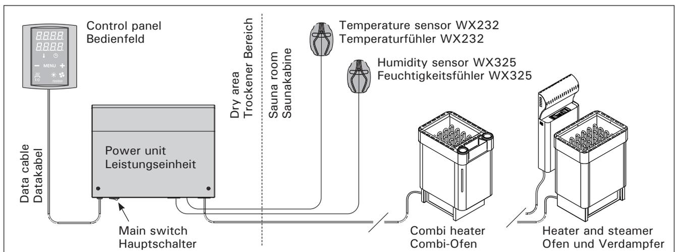
Figure 1. System components
