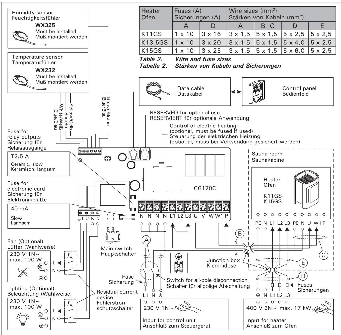
**Figure 6. Electrical connections (K11GS-K15GS)**
