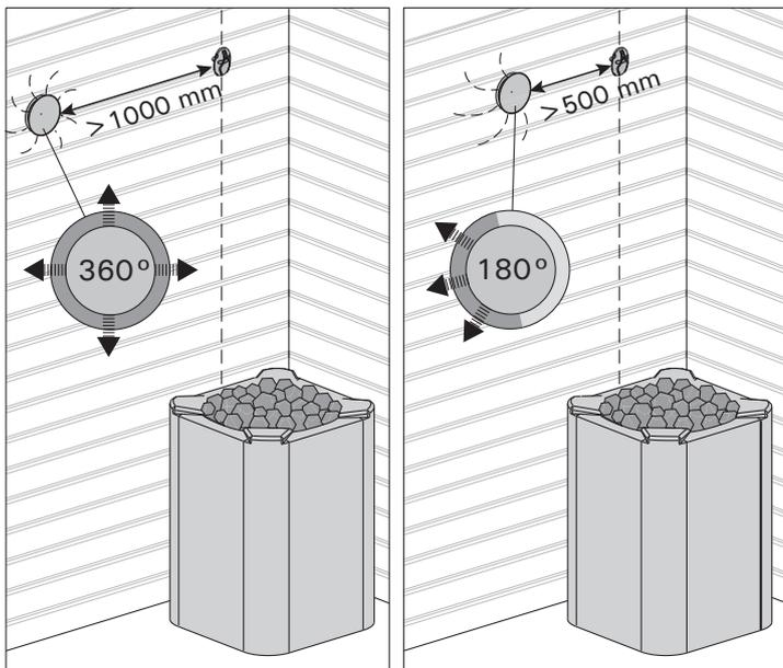
Figure 10. Sensor's minimum distance from an air vent
