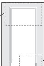
**4.** Leave a gap of about 10 mm between the upper side of the frame and the opening. It is recommended to leave 100–200 mm gap under the door for ventilation in the sauna (about 10 mm in other rooms).
