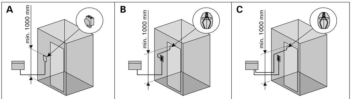
Figure 4. Options for sensor type and placement
