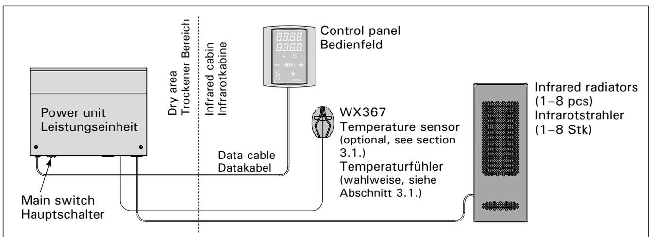
Figure 1. System components
