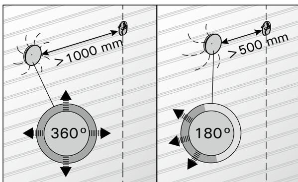
Figure 5. Sensor's minimum distance from an air vent
