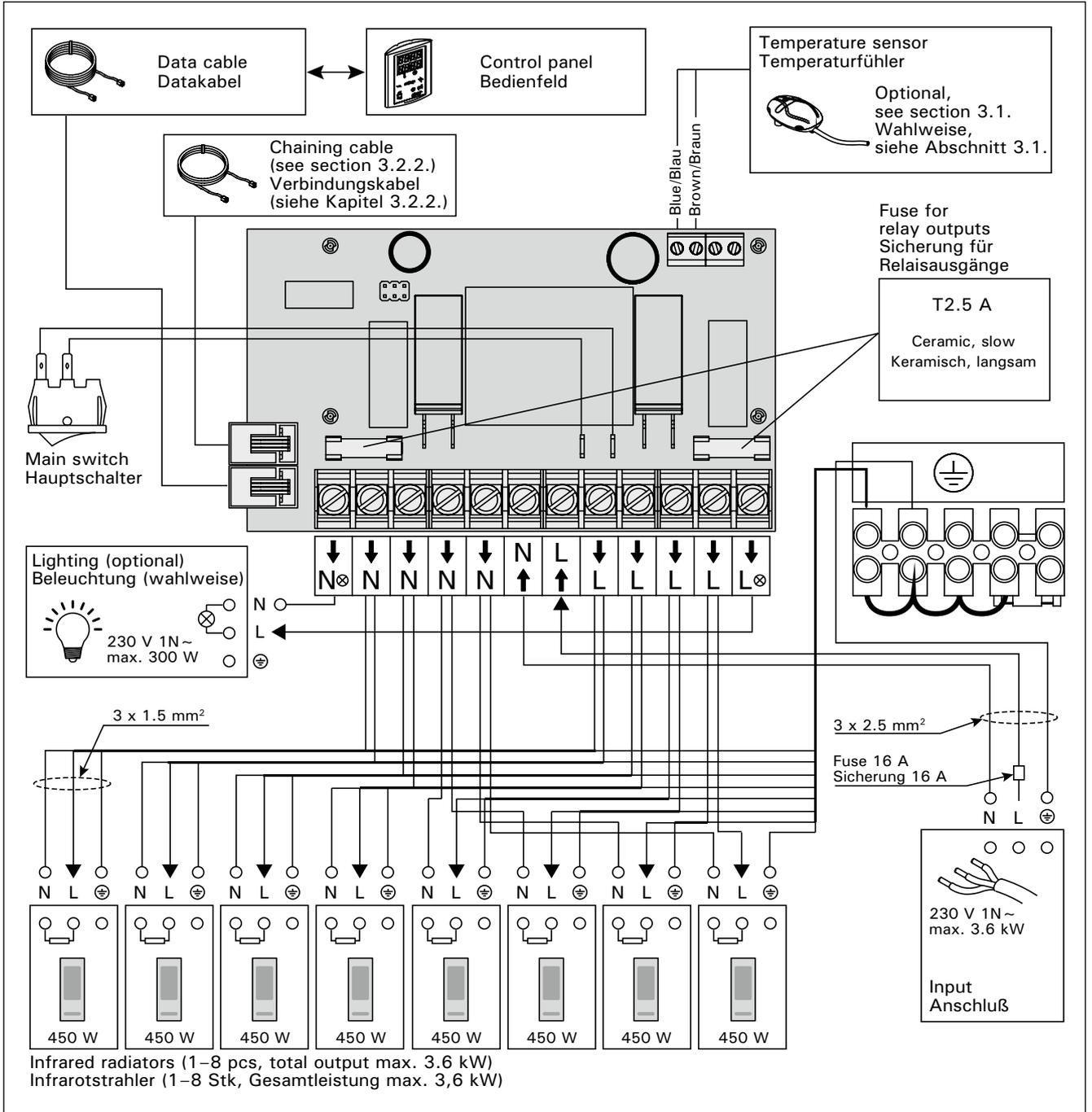
Figure 7. Electrical connections
