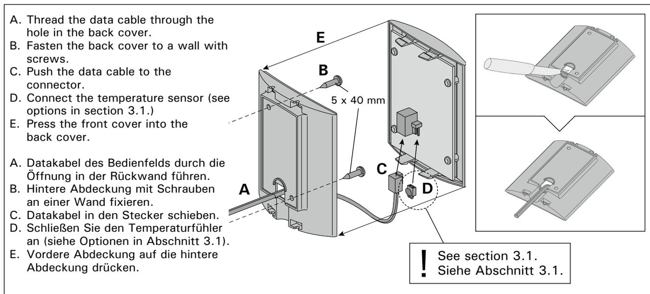
Figure 9. Fastening the control panel
